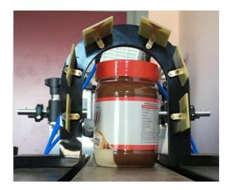
Fig. 1. Antennas array surrounding the item to inspect
