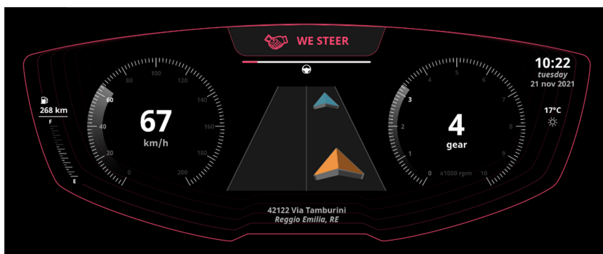
Fig. 6. Sketch of HMI for a control sharing between human driver and automated system.
