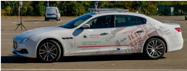
Fig. 2. Maserati prototype vehicle used by the PRYSTINE Project. The car is equipped with a range of cameras, radars, communication sensors and feedback devices, serving as a testbed for both level 2 and level 3 ADFs.
