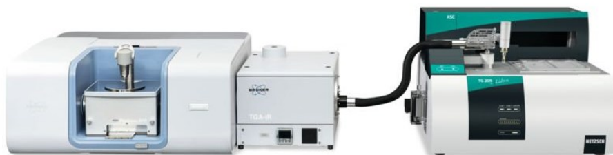
Fig. 26: TG 209 F1 Libra instrument coupled with Bruker Tensor II instrument.
