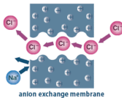
Fig. 10: AEM working principle [source: http://www.astom-corp.jp ].
