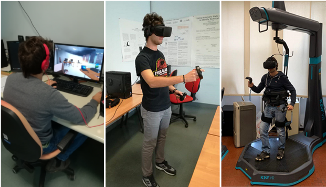
Figure 3.12: VR environments considered in this study: desktop VR (DVR, left), immersive VR (IC, center) and treadmill based immersive VR (KAT, right).
