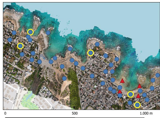
Figure 5. UAS orthoimage of the shore of Santa Sabina, with superimposed the topographic vertexes (red triangles) and the GCPs (blue dots) used for the georeferentiation of the photogrammetric flights.
