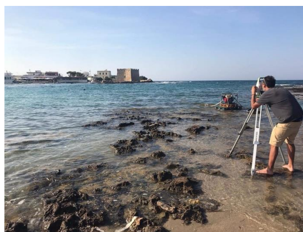
Figure 8. The image shows the topographical survey operation in Torre Santa Sabina performed to measure the position of the underwater markers.
