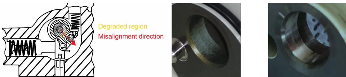
Figure 6.7: RD Control Shaft degraded surface [49]
