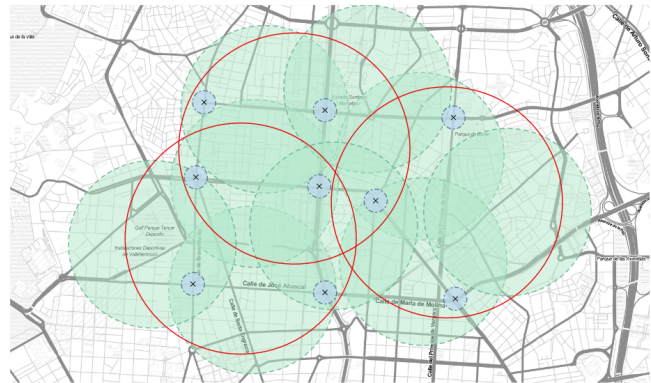
Fig. 9. Road topology used in the large-scale scenario. The nine crossings correspond to endpoints; red, green, and blue circles represent the coverage areas of macro-, micro- and pico-cells, respectively.
