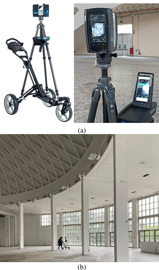
Figure 1. The components of the Swift System by FARO Technologies (a). A view of the acquisition phase in the Torino Esposizioni Hall B.
