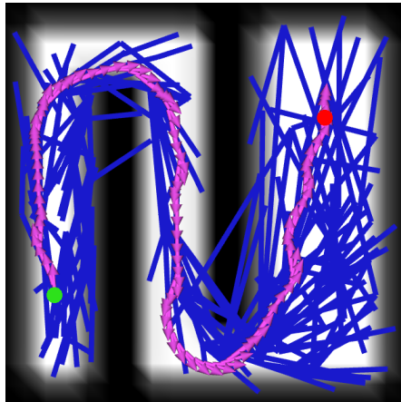
Fig. 8 Example of trajectory computed with the MP-RRT # by constructing a graph with 400 vertices. The start and target positions are in green and in red, respectively. In blue the graph \mathcal{G}^Y in the reference space, while in magenta the computed path obtained from the graph \mathcal{G}^X in the state space.
