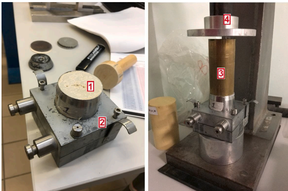
Fig. 6. Specimen of two-component grout before demoulding (left) and insertion phase of the specimen in the shear box (right). Sample held in the mould (1), Casagrande shear box (2), push cylinder (3), and pushing frame (4).
