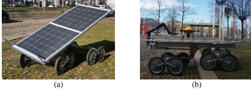
Fig. 3. Usage of the orientable upper panel during solar recharge (a) and for safe drone landing (b).
