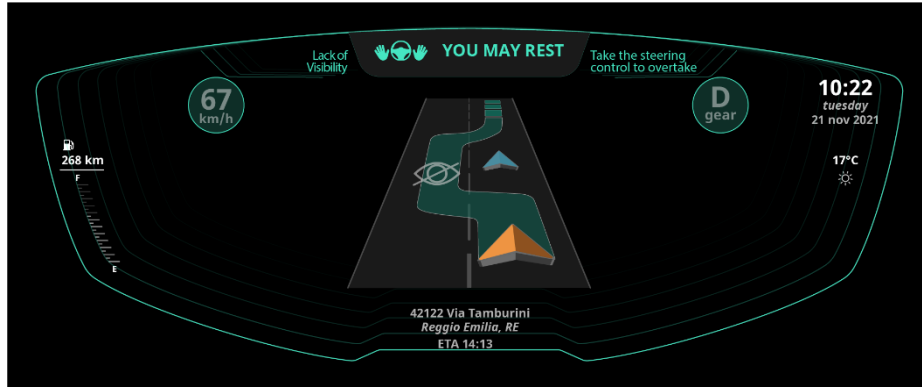
Fig. 7. Sketch of HMI informing driver about the action selected by the system (CF maneuver in this case).
