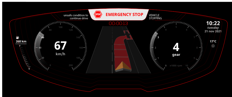
Fig. 8. Sketch of the HMI that informs the driver about the reason of the actuation for an emergency maneuver.
