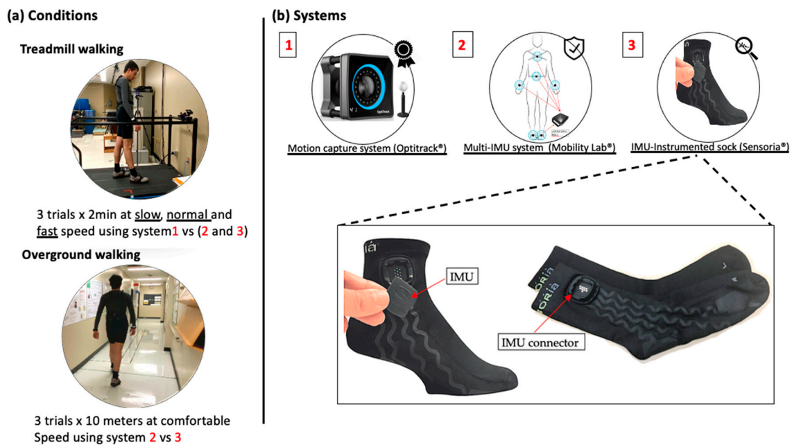
Figure 1. Conditions and measurement systems used for data acquisition. (a) Participants performed three 2 min treadmill walking trials at slow, normal, and fast walking speeds and three 10 m overground walking trials at a self-selected comfortable speed. (b) A motion capture system was used as the gold standard to validate the estimations of the spatio-temporal parameters for treadmill walking based on the IMU-instrumented sock and the Mobility Lab system.
