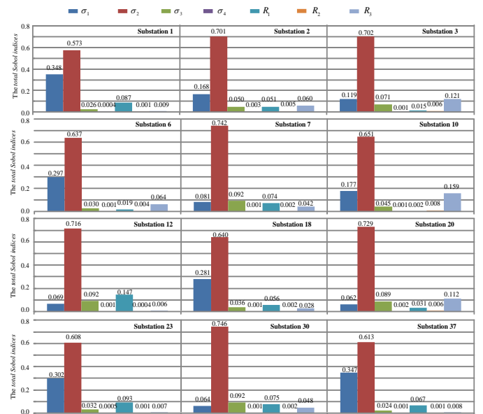
Fig. 11. The total Sobol indices of the maximums of GICs in 12 substations. \sigma_1, \sigma_2, \sigma_3, and \sigma_4 are the earth conductivities of the 4-layer model. R_1 denotes the resistance per unit length of transmission line; R_2 denotes the winding resistance.
