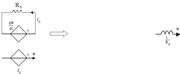
Figure 7. Coupling between magnetic and eddy current domain
