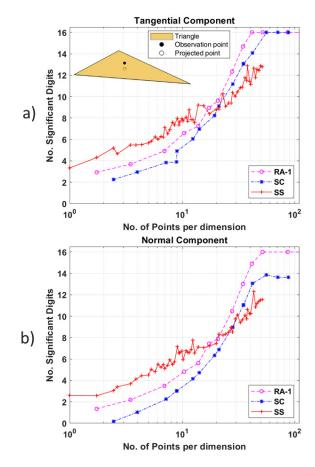
Fig. 6. No. of correct significant digits versus the no. of quadrature sample points per dimension; case of a flat triangle with observation point  $\lambda/100$  off the triangular surface projected close to the triangle centroid (inset); (a): integral tangential component; (b): integral normal component.
