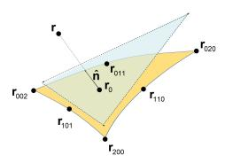
Fig. 4. Curvilinear triangle and corresponding flat tangent triangle at the projected observation point  ${\bf r}_0$ .
