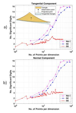
Fig. 10. No. of correct significant digits versus the no. of quadrature sample points per dimension; case of a curvilinear triangle with observation point  $\lambda/100$  off the triangular surface projected close to the triangle centroid (inset); (a): integral tangential component; (b): integral normal component.
