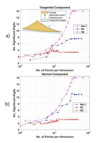
Fig. 12. No. of correct significant digits versus the no. of quadrature sample points per dimension; case of a curvilinear triangle with observation point  $\lambda/100$  off the triangular surface projected on one triangle edge (inset); (a): integral tangential component; (b): integral normal component.
