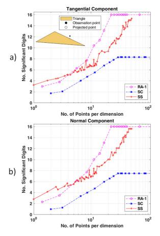
Fig. 8. No. of correct significant digits versus the no. of quadrature sample points per dimension; case of a flat triangle with observation point  $\lambda/100$  off the triangular surface projected on one triangle edge (inset); (a): integral tangential component; (b): integral normal component.
