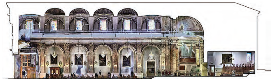
Fig. 1. Lateral section of the church obtained from the point cloud of the laser scanner survey.
