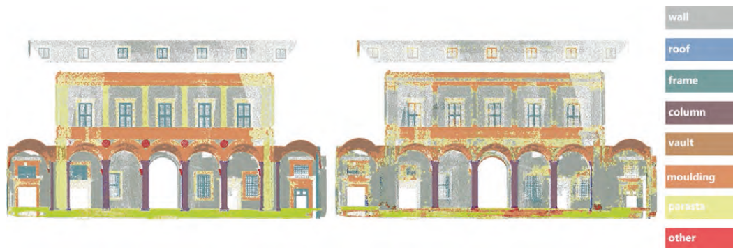
Fig. 4. Qualitative results about the segmentation of point clouds for the Ducal Palace.
