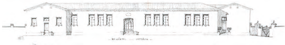
Fig. 1. Ex Mercato di Torre Spaccata, side elevation: overlaying of the original project drawing on the orthophotoplan from point cloud.
