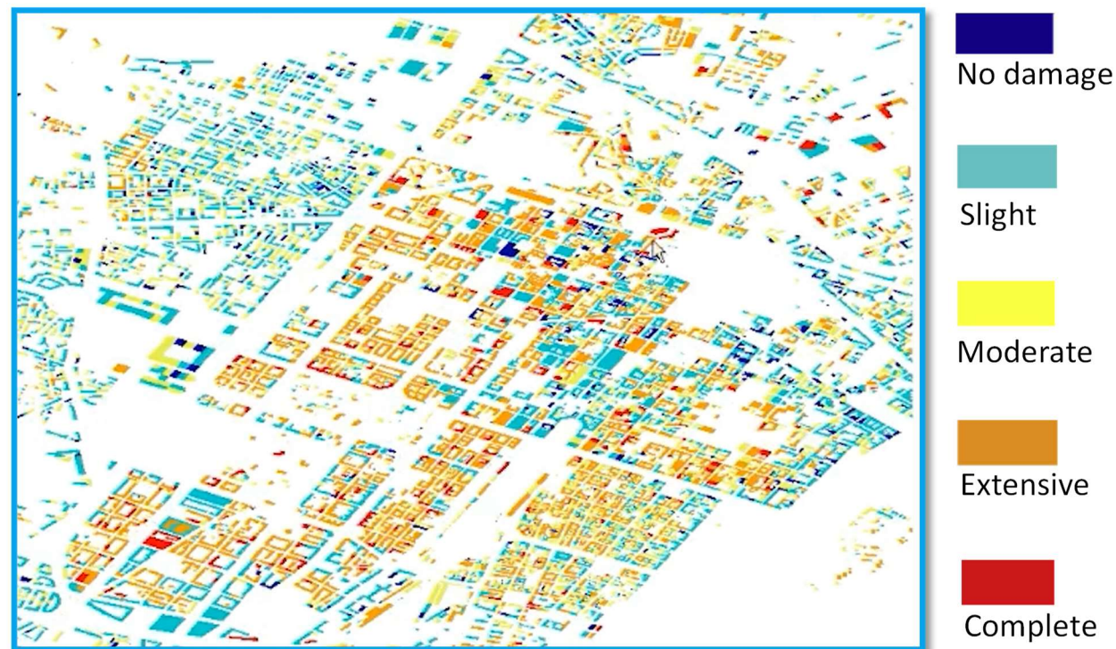
Figure 1. Integrated platform by (Marasco et al., 2021a): (a) seismic scenario selection, (b) building damage visualization on the IdealCity computed by the surrogate physical model (Marasco et al., 2021b).
