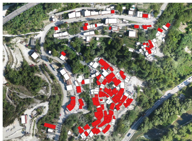
Figure 4. The image shows the damage classification performed by DEEP on the Pescara del Tronto 2016 orthophoto, using the Mozambique classification model. The not-affected buildings are marked in white, while the damaged buildings are marked in red colors.
