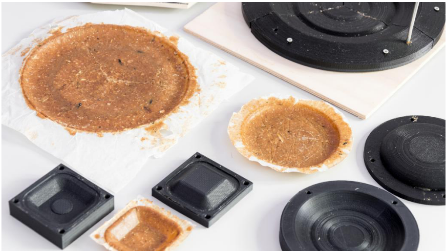
Figure 5. Set of PLA moulds used to give shape to the vegetable polymer.
