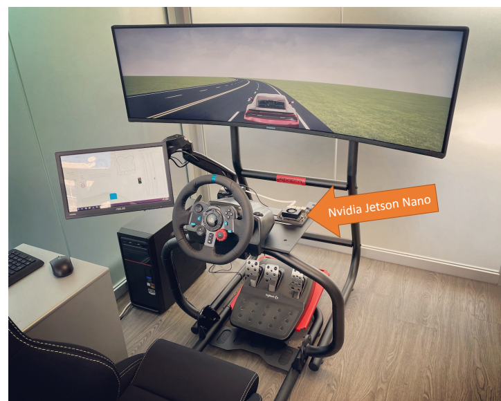
Figure 8. Hardware-in-the-loop (HIL) simulation.
