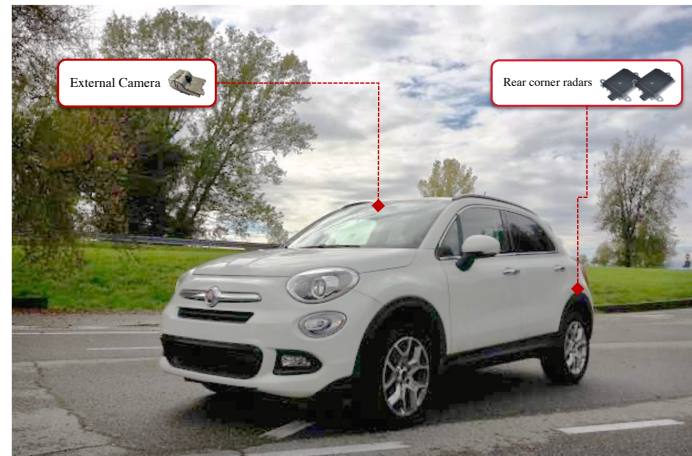
Figure 2. Prototype vehicle with installed sensors.
