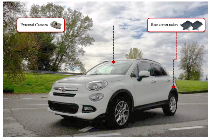
Figure 2. Prototype vehicle with installed sensors.
