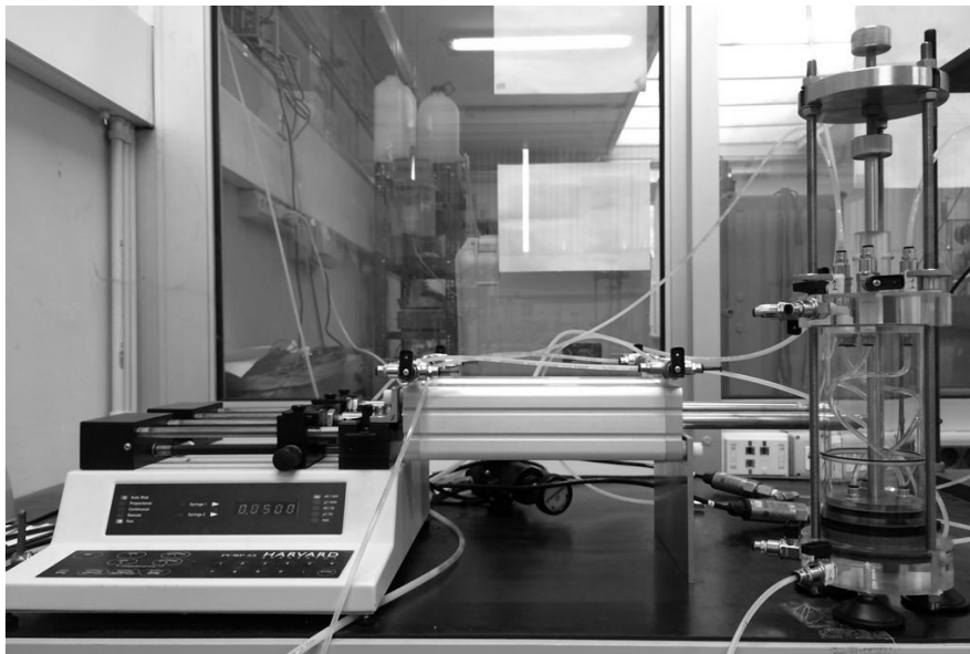
Figure 3. Pictorial view of the chemico-osmotic testing apparatus.
