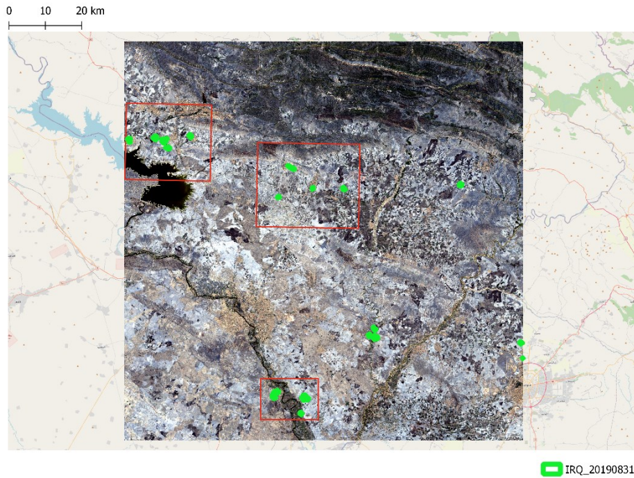
Figure 3.13 Map showing Sentinel-2 image tested in this exercise, IDP camps belonging to the collected dataset (in green) and sub-areas selected for the training and testing (in red).
