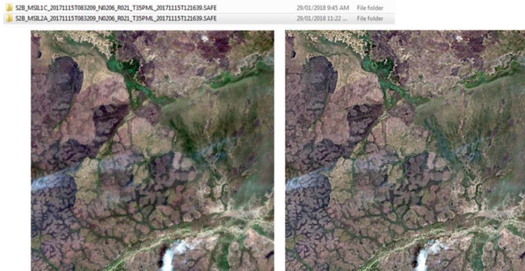
Figure 5.14 Effect of the application of the Sen2Cor processor over a Sentinel-2 L1C product (left) generating a Sentinel-2 L2A product (right).
