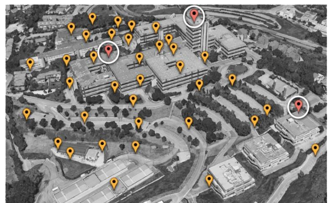
Figure 10. The simulated scenario with three GWs located in the campus area: hot spots (yellow markers) and GWs (white circled red markers) placement.
