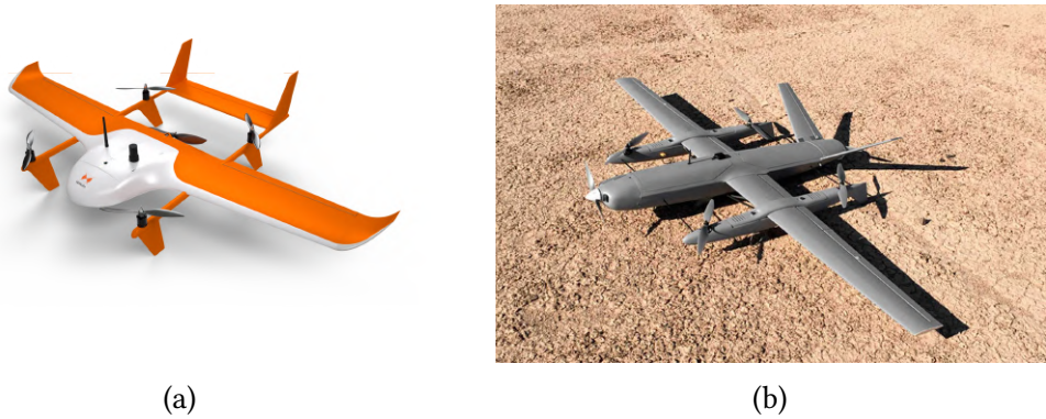
Figure 1.3: hybrid VTOL-fixed wing drones Foxyslim [133] in Fig.1.3a and Pelican [67] in Fig.1.3b.
