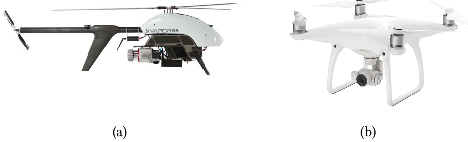
Figure 1.5: two different types of rotary-wing drone; Fig.1.5a shows the helicopter-like Vapor [16] while Fig.1.5b shows the quadrotor Phantom 4 [95].
