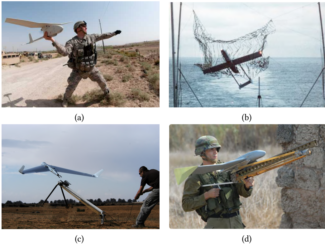
Figure 1.2: manual launch of ‘Raven RQ-11B’ [20] in Fig.1.2a, a recovery net on the stern of a battleship catches a Pioneer I [243] in Fig.1.2b, the launch catapult of the ‘Orbiter’ [18] in Fig.1.2c, and the manual launch catapult of the ‘BlueBird’ [53] in Fig.1.2d.
