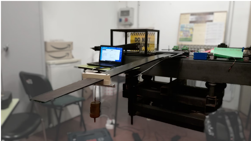
Figure 4.33: Experimental setup for the static loading test on the wing
