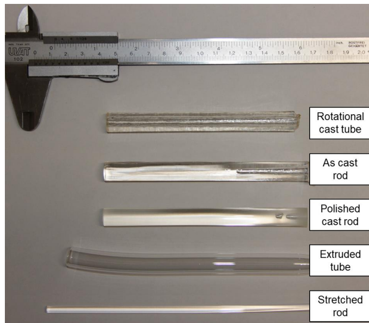
Fig. 3. Examples of core and cladding glass preforms used for the fabrication of the optical fibers: rotational casting cladding tube, as-cast and polished core rod, extruded cladding tube, and stretched core rod.
