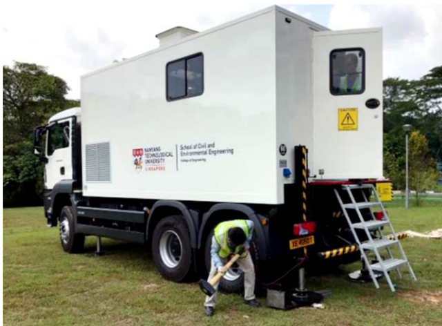
Figure 3. GEM3 mobile station for rapid geotechnical, environmental and traffic monitoring and testing developed at Nanyang Technological University, Singapore
