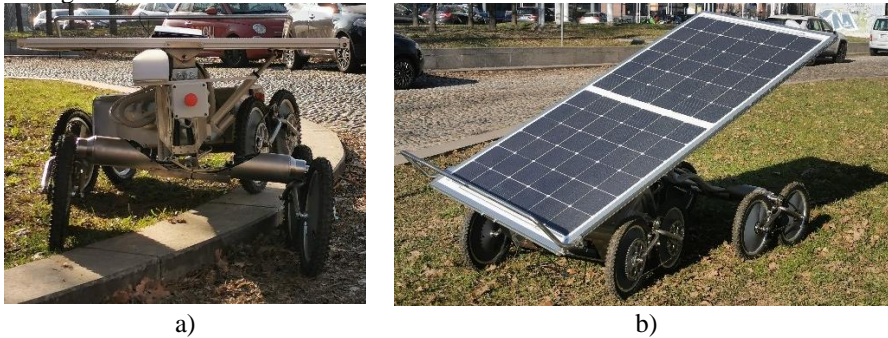
Fig. 3. a) Landing platform; b) solar panels.
