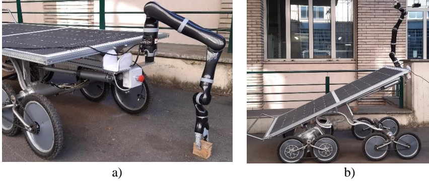
Fig. 4. a) The End effector of the robotic arm reaches the ground; b) end effector maximum height.
