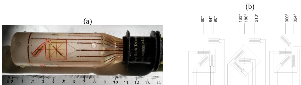
Figure 1. (a) photo illustration of a Hollow Inclusion cell (HI cell) with the prominent four electrical strain gauge oriented in different directions. Some electrical connections between the individual strain gauges and the multipolar cable connecting the strain gauges and the Wheatstone bridge generally used for carrying out the measurements are also visible; (b) schematic representation of the distribution of strain gauge sensors along the median section of the HI cell's circumference.
