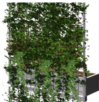
Fig. 9 Vases with metal support for climbing plants
