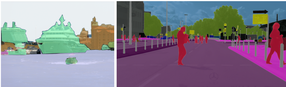
Figure 2.3: Examples of semantic segmentation for COCO [76] (left) and Cityscapes [28] (right) datasets.
