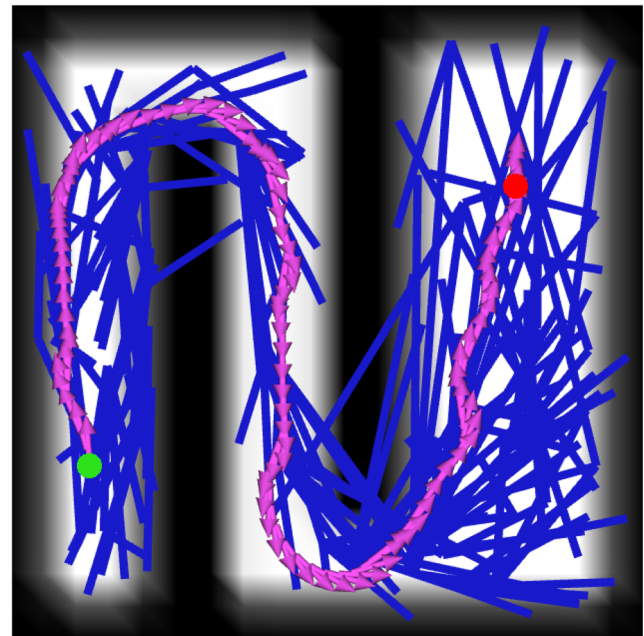
Fig. 8 Example of trajectory computed with the MP-RRT # by constructing a graph with 400 vertices. The start and target positions are in green and in red, respectively. In blue the graph \mathcal{G}^{\mathcal{Y}} in the reference space, while in magenta the computed path obtained from the graph \mathcal{G}^{\mathcal{X}} in the state space
