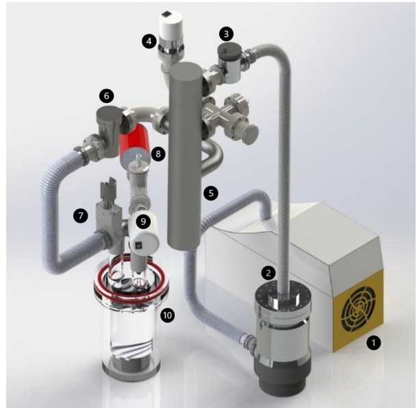
Figure 3: Launch volume/test section, subsystem 200. 1: Roots pump. 2: Turbomolecular pump. 3: Bellows sealed valve. 4: Full range pressure transducer. 5: Launch volume. 6: Bellows sealed valve. 7: Gate valve. 8-9: Capacitive pressure transducers. 10: Test section.
