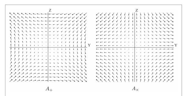
**Figure 2.** The gravito-magnetic field **B**: on the left, we suppose that the GW has just the  $A^+$  polarisation; on the right, we suppose that the GW has just the  $A^+$  polarisation. Notice that the two polarisations differ by a rotation of  $\pi/4$ .
