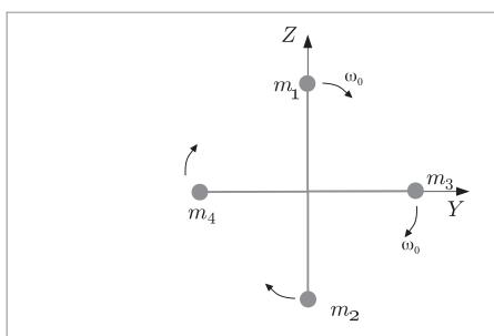
**Figure 3.** Two identical dumbbells are made by test masses  $m_1=m_2=m_3=m_4=m$  at fixed distance R, and rotated by  $\pi/2$  with respect each other. They independently rotate with frequency  $\omega_0$ , before the passage of the wave.
