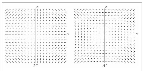
**Figure 1.** The gravito-electric field **E**: on the left, we suppose that the GW has just the  $A^+$  polarisation; on the right, we suppose that the GW has just the  $A^\times$  polarisation. Notice that the two polarisations differ by a rotation of  $\pi/4$ .
