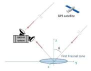
Figure 1. GNSS-R measurements system.
