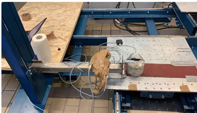
Fig. 2 – Shaking table test setup
