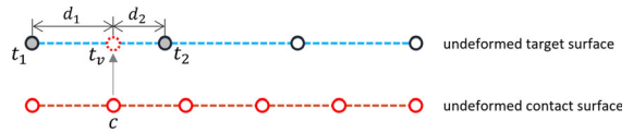
Fig. 6 The contact node c is projected onto the target interface, so that the virtual node t_v is found and the corresponding target nodes t_1 and t_2 are identified
