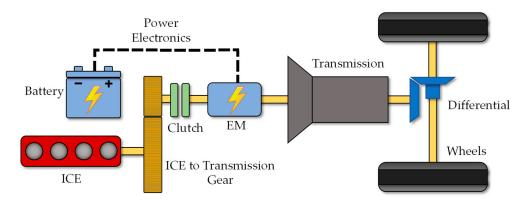
**Figure 1.** Parallel P2 full hybrid electric vehicle (HEV) architecture.
