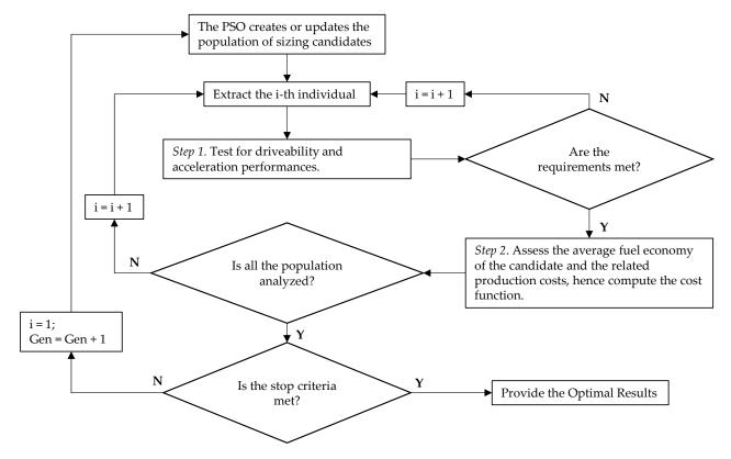
Figure 2. Complete design workflow.
