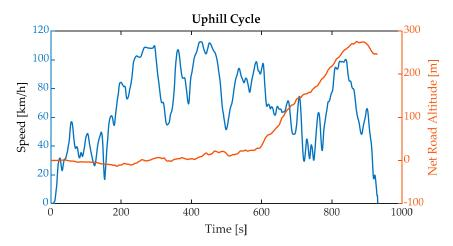
Figure 4. Speed profile and net road altitude variation of the uphill real-world drive mission.
