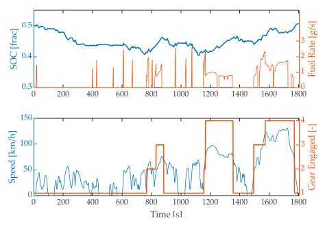
**Figure 7.** Example of the DP control results for a four-speed HEV driving the WLTP, equipped with a 99 kW ICE and a 29 kW EM.
