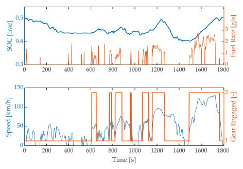
**Figure 6.** Example of the DP control results for a two-speed HEV driving the worldwide harmonised light vehicles test procedure (WLTP), equipped with a 68 kW ICE and a 14 kW EM.
