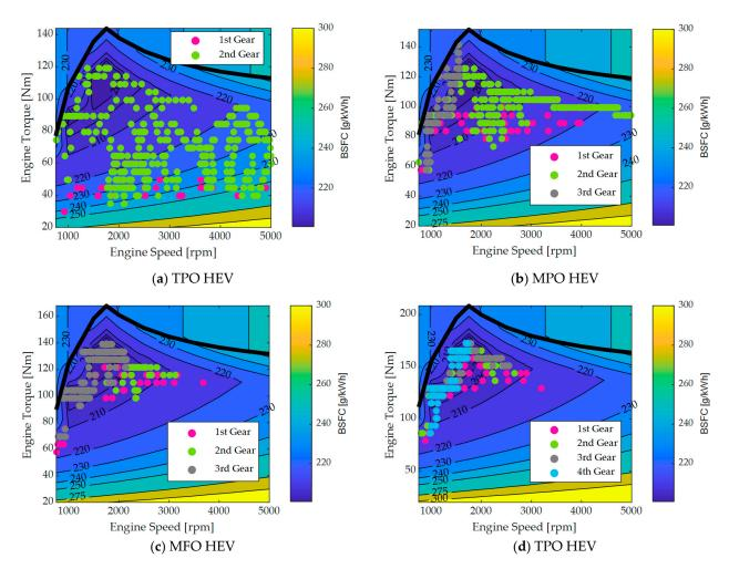
**Figure 9.** ICE operating point obtained in the WLTP drive mission for the (a) totally production-oriented, (b) mostly production-oriented, (c) mostly fuel-oriented, and (d) totally fuel-oriented optimal layouts. The colored map shows the brake specific fuel consumption (BSFC) areas, whereas the solid black line instead is the WOT curve.
