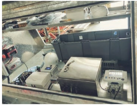
Figure 2. Interior spacing of the trailer, showing the wet area, communications box and sensor equipment.
