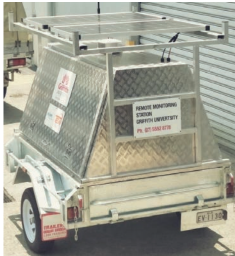
Figure 1. Trailer exterior modified with solar panels.
