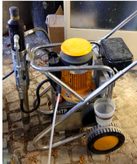
Fig. 5. One-component injection piston pump Taiver HTP 210000 used for the sample grouting.
