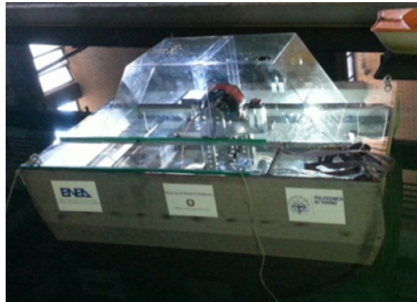
Figure 3. Photo of the 1:12 PeWEC prototype tested in a wave tank [31].
