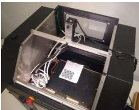
Figure 1. Printer setup with the Svpro camera and checkerboard pattern.
