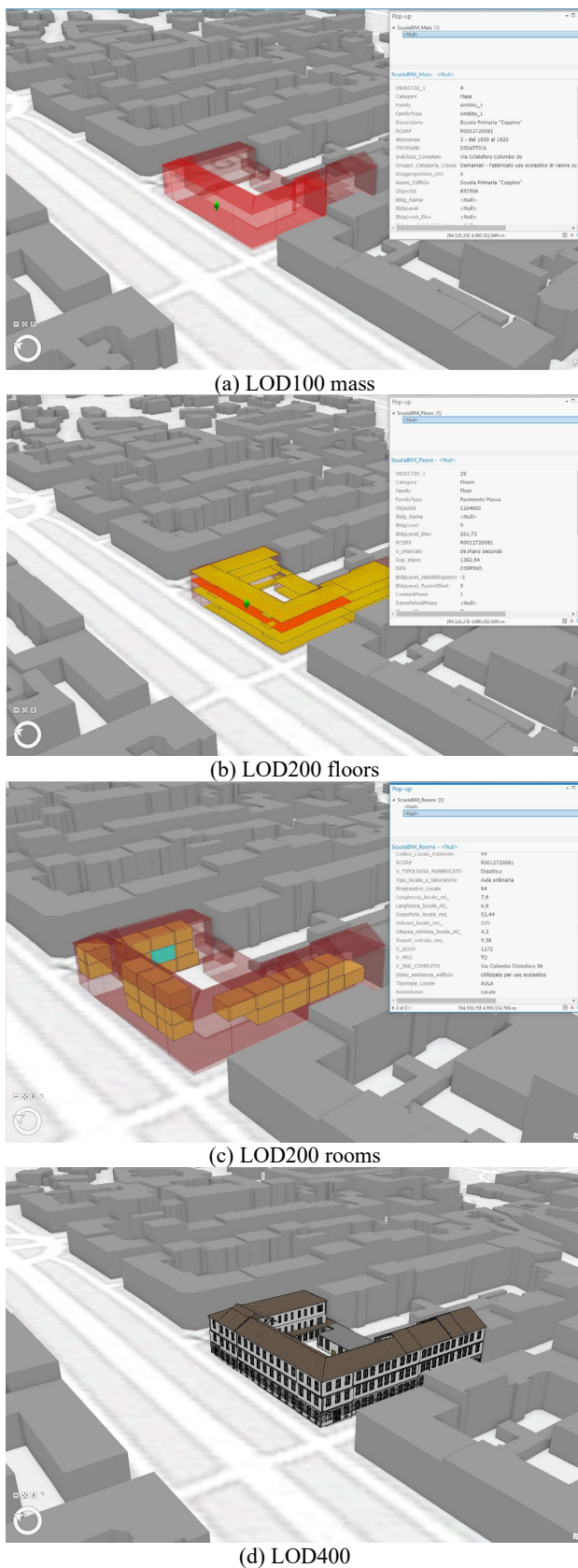
Figure 9. The Scuola Coppino multi-scale parametric model migrated into the Digital Twin at different LODs
