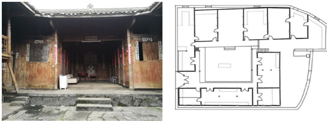
Figure 42: Photo and planimetry of a Bucket House in Yunshe. Source: photo and drawing by author according to the field survey in May 2018
