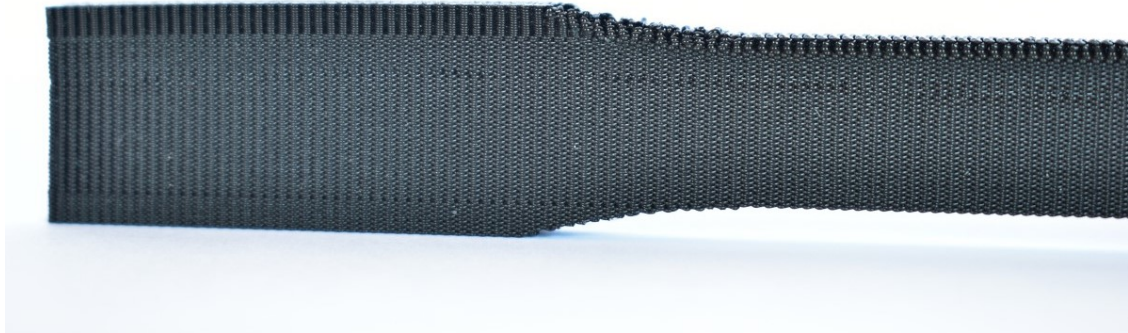
Figure 3.15: Magnified view of the printing defects in a dog-bone specimen for direction 2.
