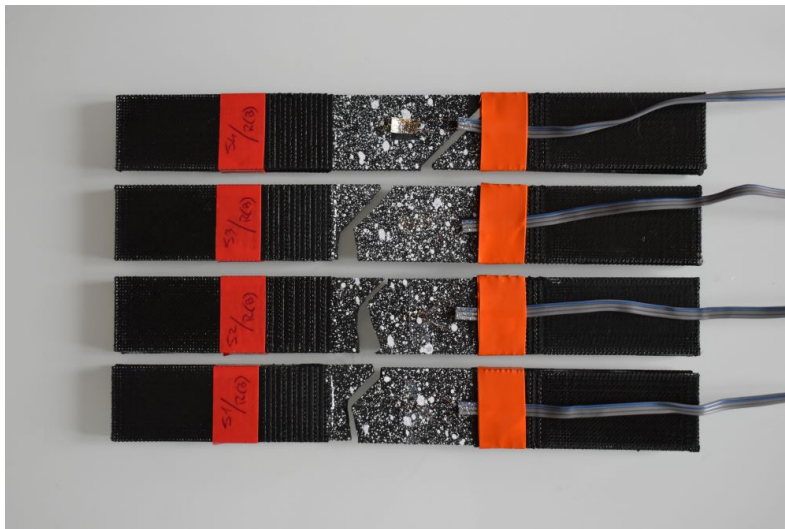
Figure B.10: Failure modes of Run(I) specimens.
