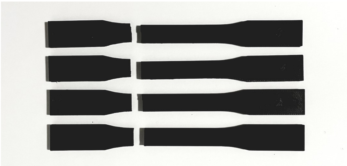
Figure 3.13: Failed dog-bone specimens for mechanical properties evaluation in direction 1 after the preliminary tests.
