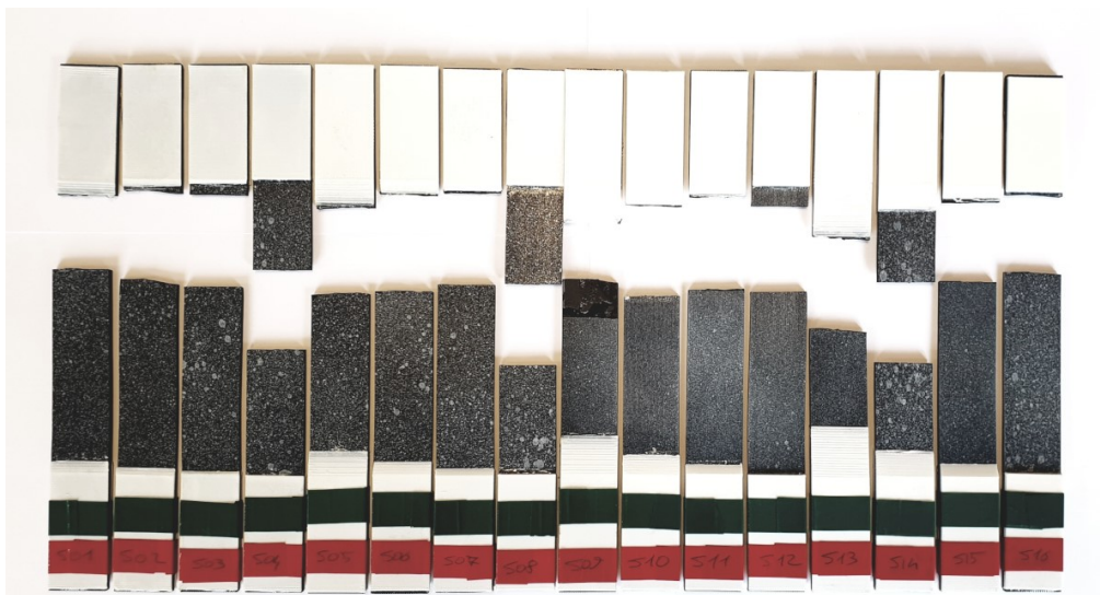
Figure 3.21: First DoE, tensile specimens loaded in direction 1 after the tests.
