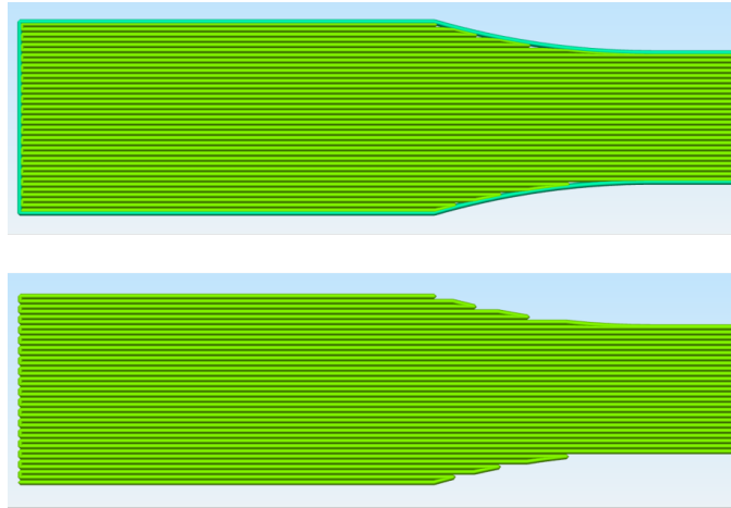
Figure 3.10: Alternative printing configurations for preliminary dog-bone specimens: tensile properties determination in direction 1.
