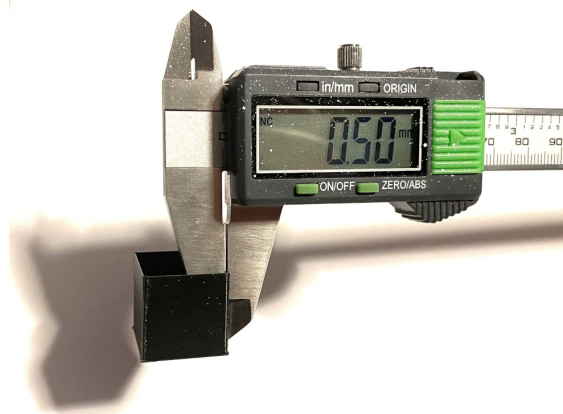
Figure 1.11: Thin wall test for extrusion multiplier quantification: the thickness of the wall should coincide with the bead width.
