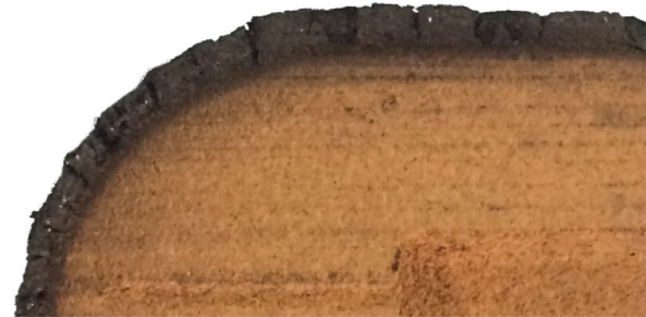
(c) Section of a P50 sample after a test in Plasmatron conducted by Sakraker [8].
