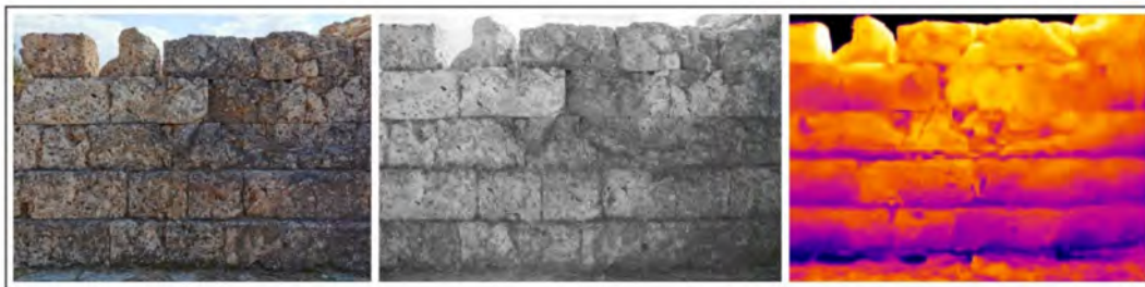
Figure 17. Reflectance images captured at the archaeological site of Lepreum: (from left to right) visible-spectrum, near-infrared, and a thermal-infrared image.
