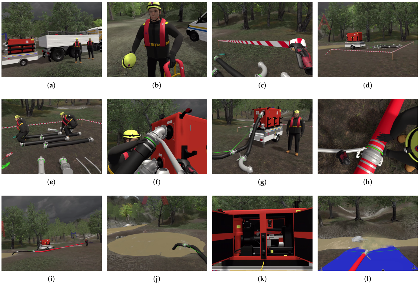
Figure 2. Excerpt of few key moments of the arranged training procedure in the VRMT. In order: arrival at the deluged area (a), an operator wears the PPE (b), delimitation of the operational field (c), final operational field (d), two operators transporting a semi-rigid tube (e), assembly of tubes using hooks and levers (f), assembly of the delivery chain (g), assembly of two foldable hoses (h), overview of the two chains (i), immersion of the filter (j), checking of the filter and impeller valves (k), discharging of water in the delivery area (l).
