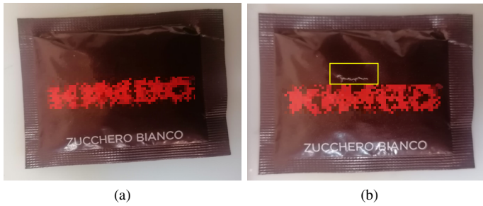
Fig. 6: Sugar bags (a) Standard packaging; (b) Defect packaging highlighted in the yellow box.
